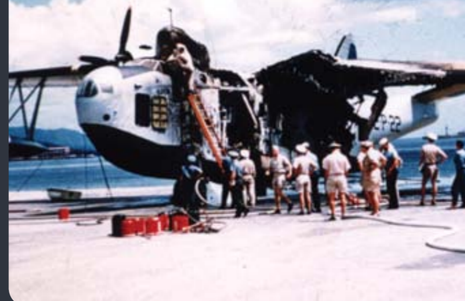
Argentinean 2-P-22 at Trinidad U.S. Naval Air Station after being damaged by a fire. Fire was caused by a back-fire of a newly installed engine during start up! The plane was damaged beyond repair and scrapped
