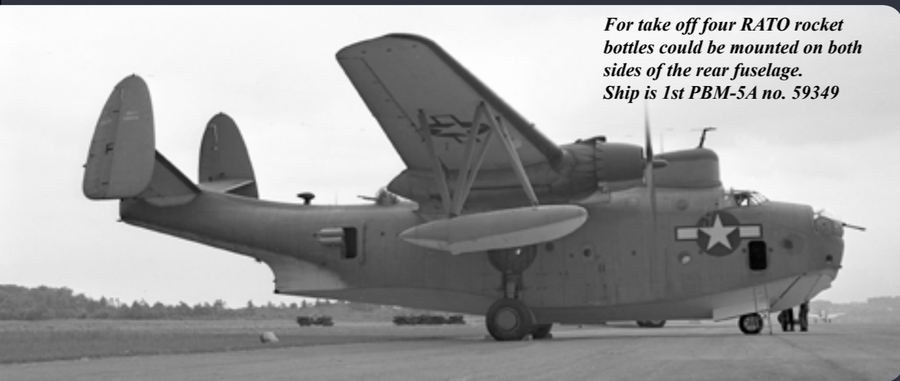
U.S. Navy PBM-5A amphibian with the nose turret and other armament removed. It is BuAer No. 122081. It became later MLD no. 16-301
