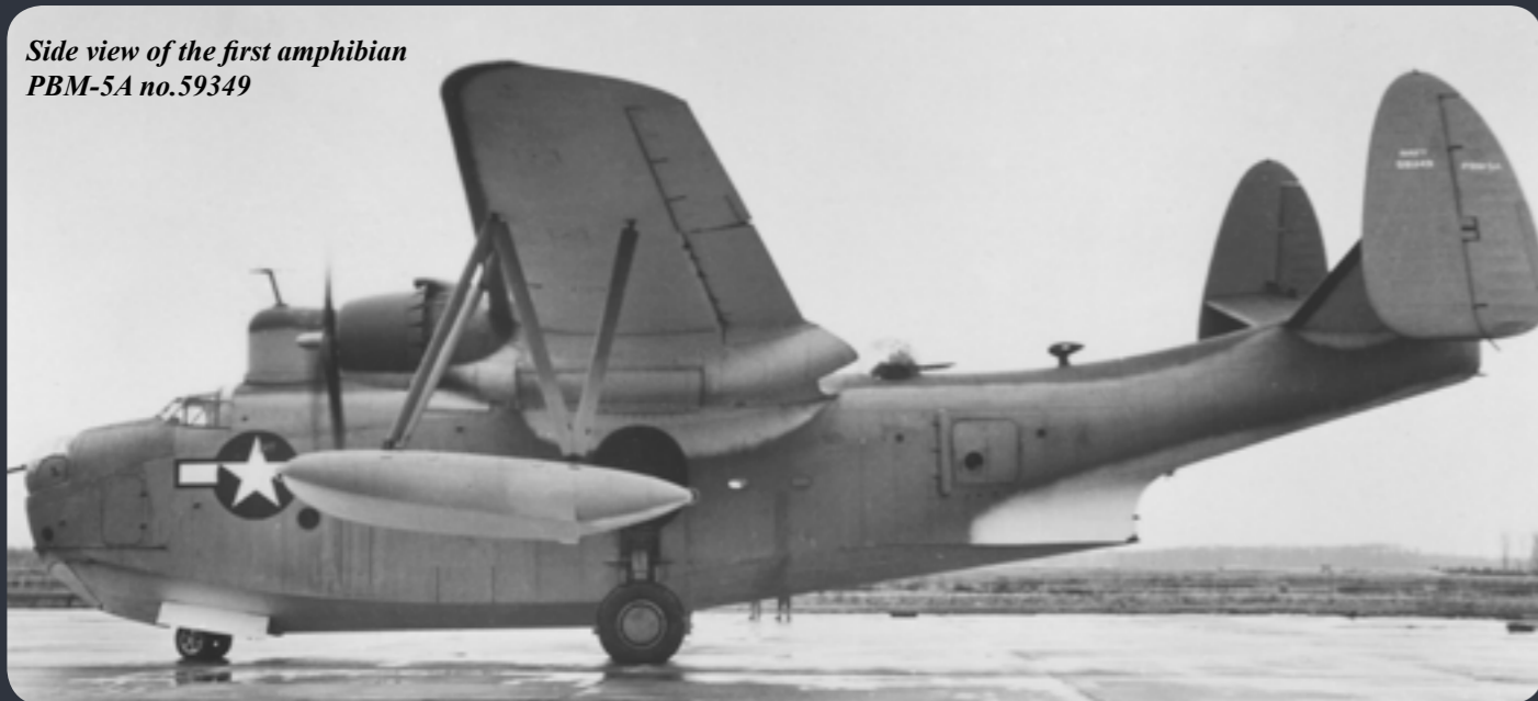
For take off four RATO rocket bottles could be mounted on both sides of the rear fuselage. Ship is 1st PBM-5A no. 59349
