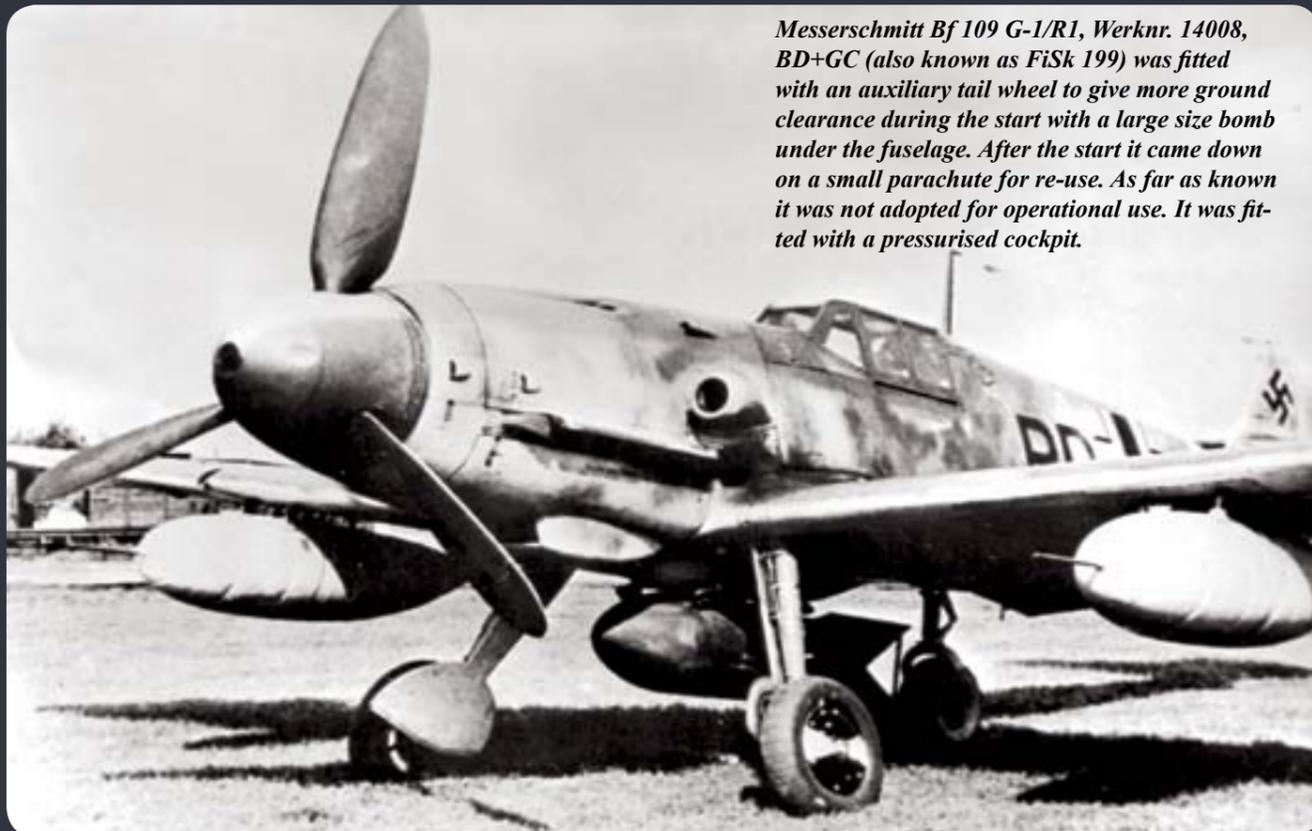
*Messerschmitt Bf 109 G-1/R1, Werknr. 14008, BD+GC (also known as FiSk 199) was fitted with an auxiliary tail wheel to give more ground clearance during the start with a large size bomb under the fuselage. After the start it came down on a small parachute for re-use. As far as known it was not adopted for operational use. It was fitted with a pressurised cockpit.*
