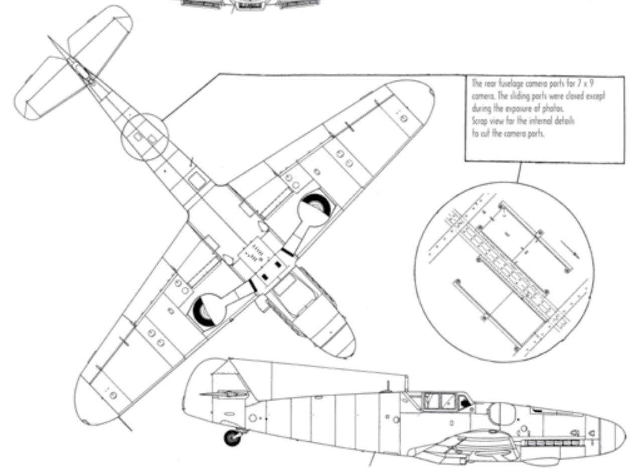
The rear fuselage camera parts for 7 x 9 camera. The sliding parts were closed except during the exposure of photos. Scrap view for the internal details to cut the camera parts.
