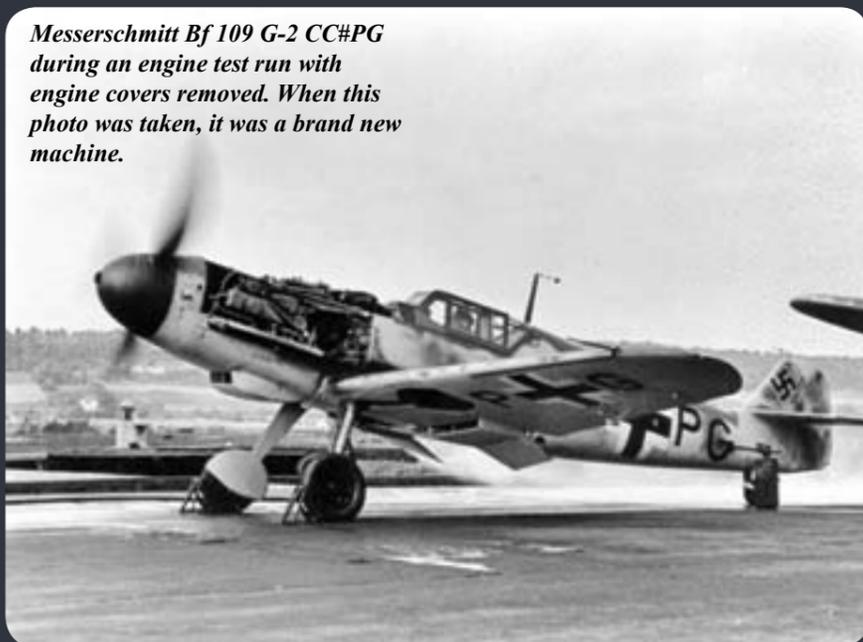
Messerschmitt Bf 109 G-2 CC#PG during an engine test run with engine covers removed. When this photo was taken, it was a brand new machine.
