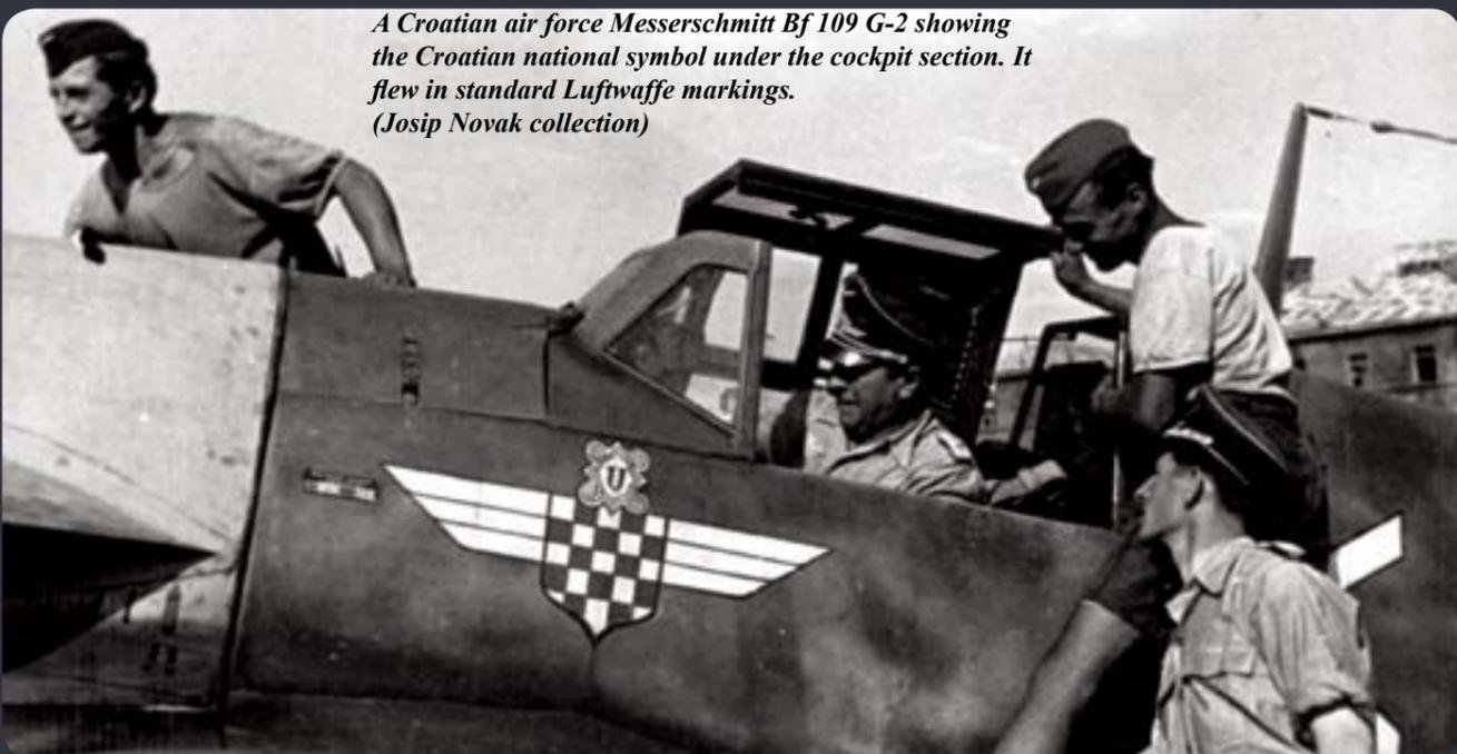
A Croatian air force Messerschmitt Bf 109 G-2 showing the Croatian national symbol under the cockpit section. It flew in standard Luftwaffe markings. (Josip Novak collection)
