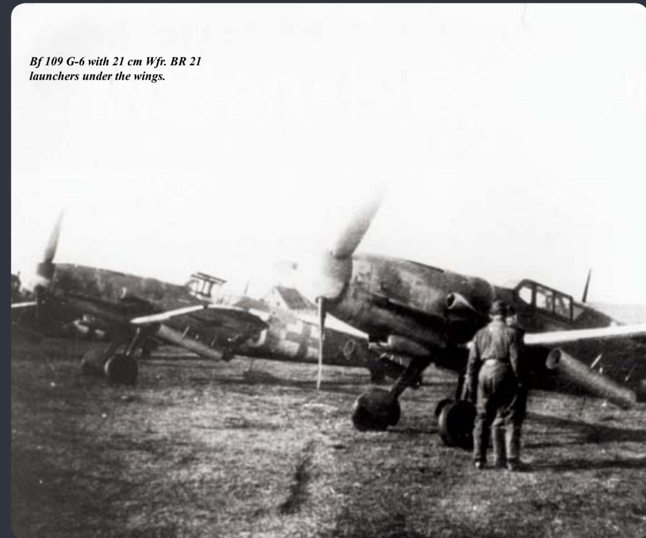
Bf 109 G-6 with 21 cm Wfr. BR 21 launchers under the wings.
