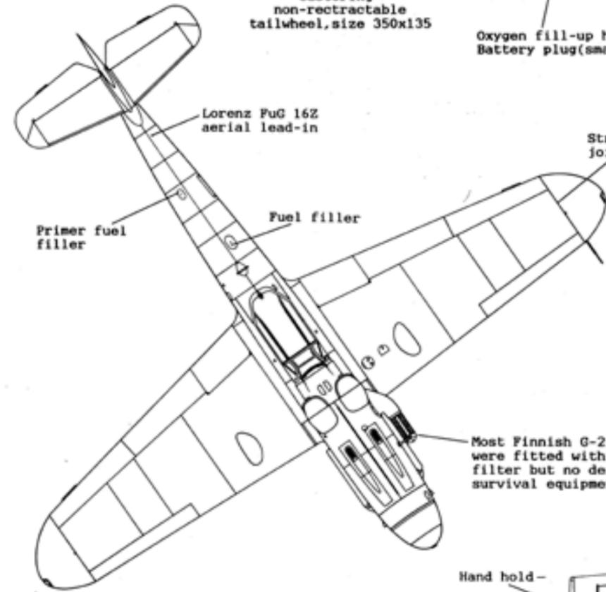
Stripe of doped fabric sealing this joint (upper and undersides)
