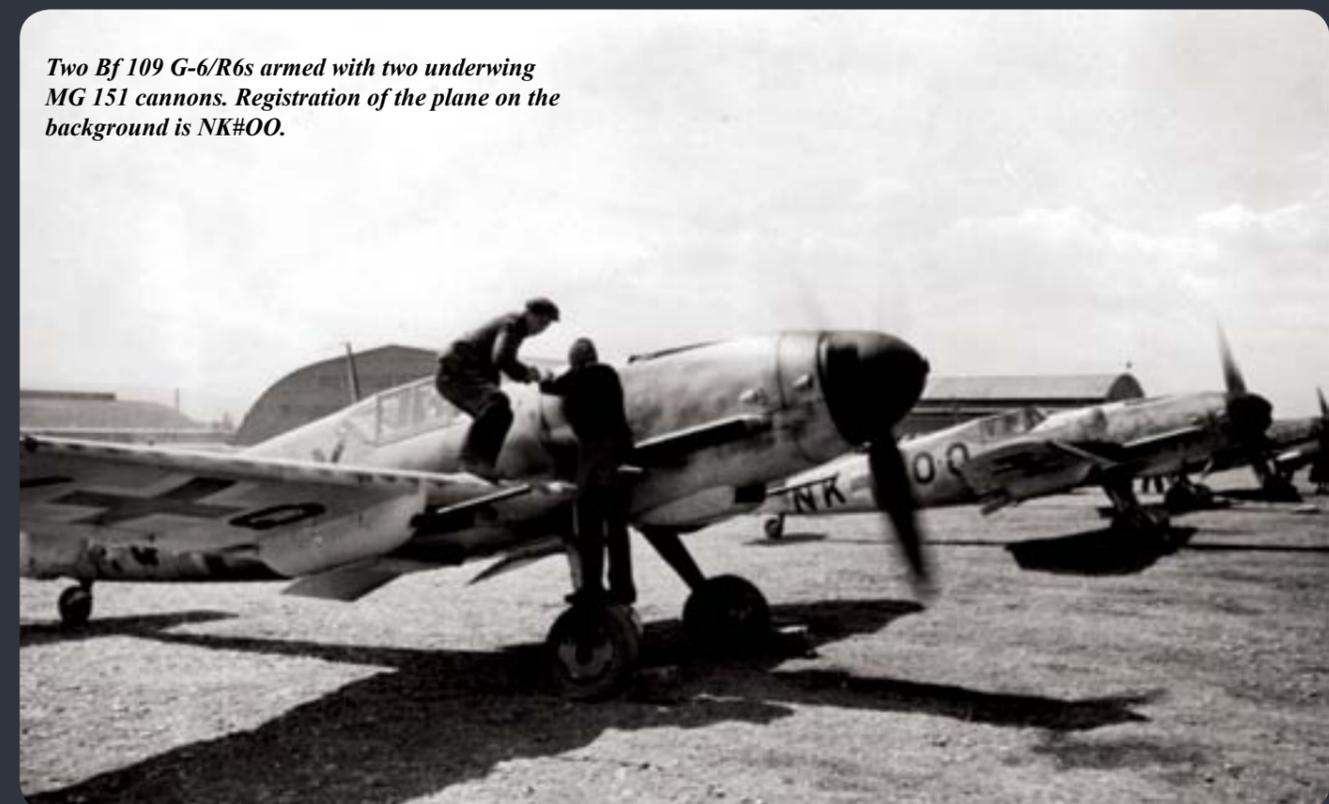
Two Bf 109 G-6/R6s armed with two underwing MG 151 cannons. Registration of the plane on the background is NK#00.
