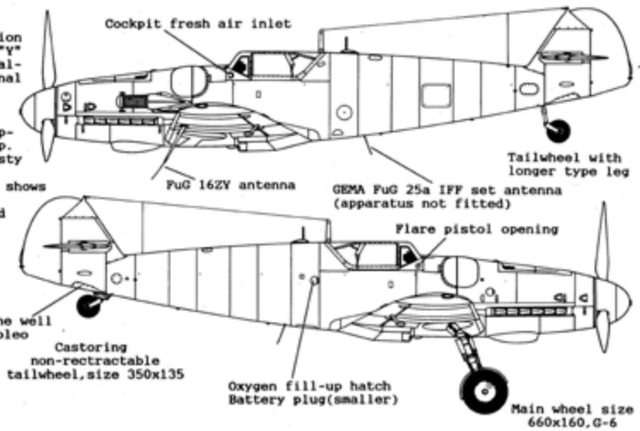
A metal plate covering the well and a dust cover on the oleo
